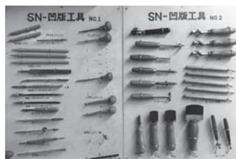
*Photo 18: Intaglio printmaking tools at Kawalabo; engraving needles, scrapers, burnishers, mezzotint rockers, roulette wheels etc.*
