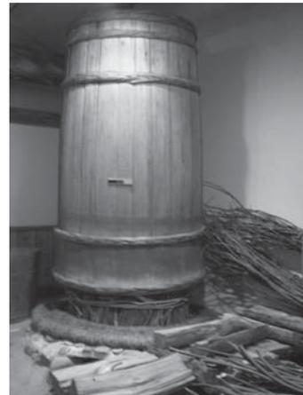
*Photo 34: Large vat to boil the tree barks in the Japanese papermaking process*
