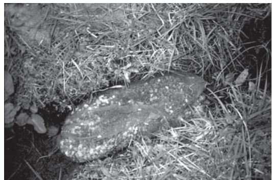
Figures 5: Zeolite, a rock-shaped mineral, is used to trap cesium in natural waterways in Nihonmatsu, Fukushima.
